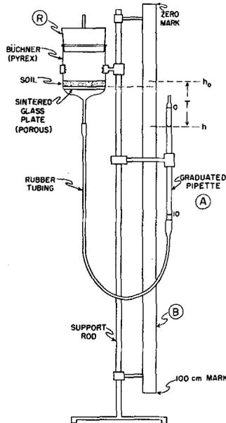
FIGURE 1. — Suction filter apparatus.
